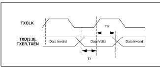
Figure 15. MII Transmit Timing Parameters
